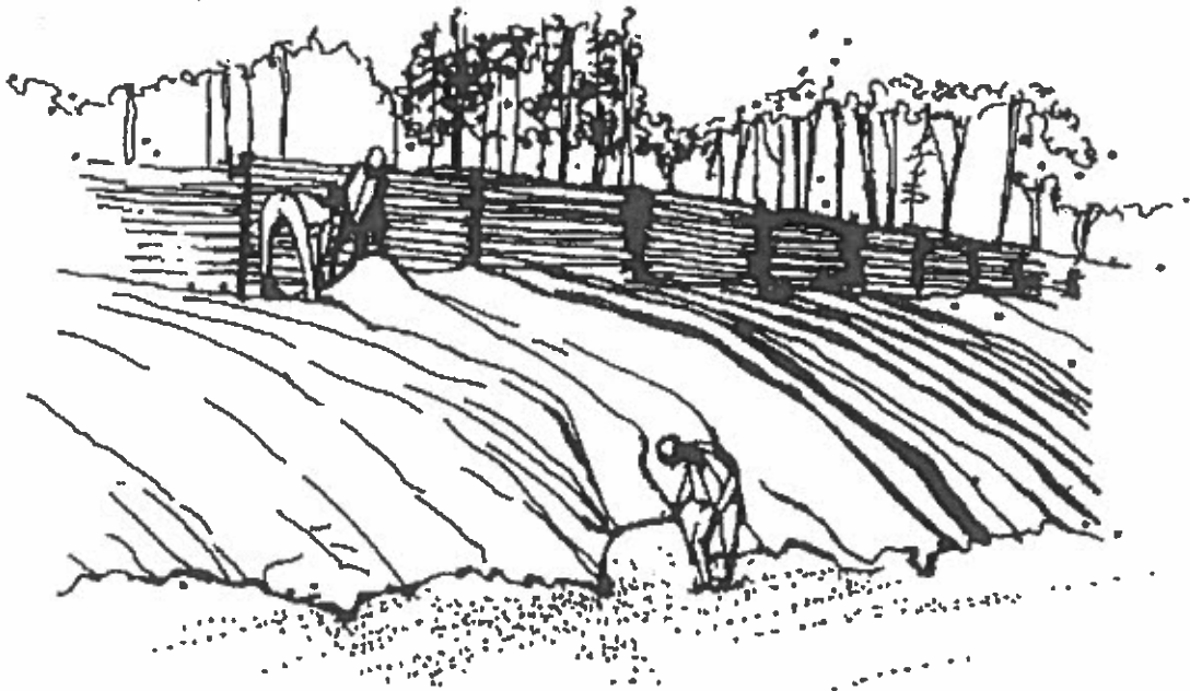
Installation of Erosion Control Blanket Perspective View
