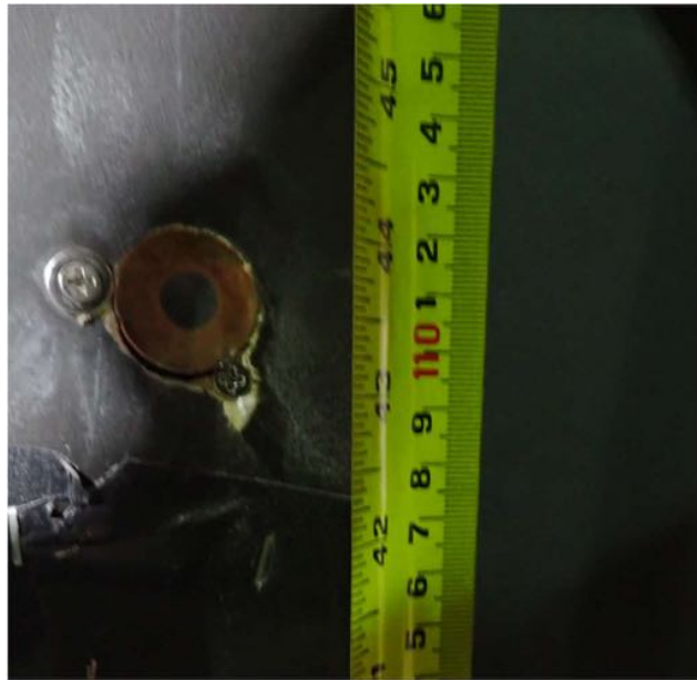
Figure C9 – Heat Flux Heat Flux Installed in the Side Wall at Mid-Unit Height
