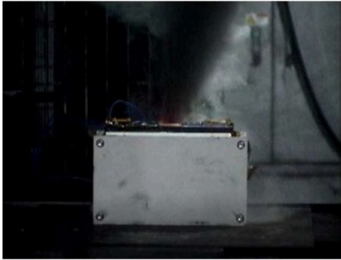
Cell 1 - Immediately before thermal runaway* (00:43:54)
