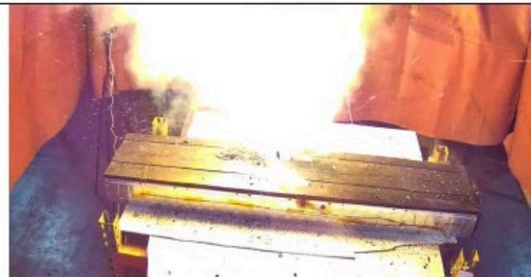
(h) Second propagation After Initiating Cell (Cell 31) 1:13:49
