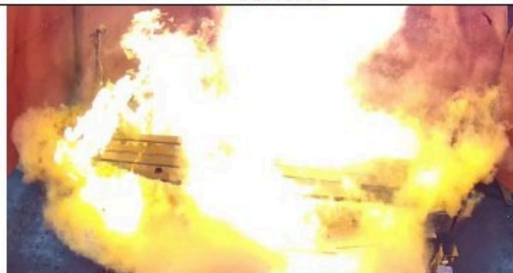
(e) Continuation of Initiating Cell Thermal Runaway 00:46:18
