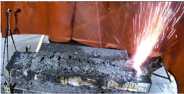
(k) Continued Thermal Runaway 04:35:51
