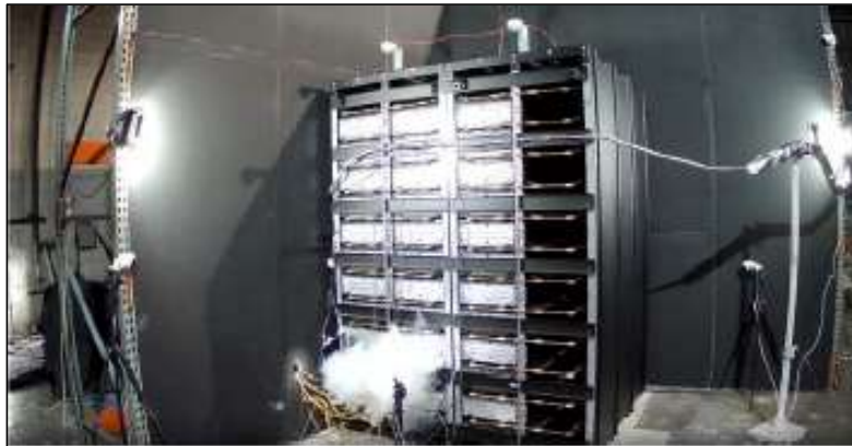
(c) Initiating Unit Thermal Runaway [00:42:25]
