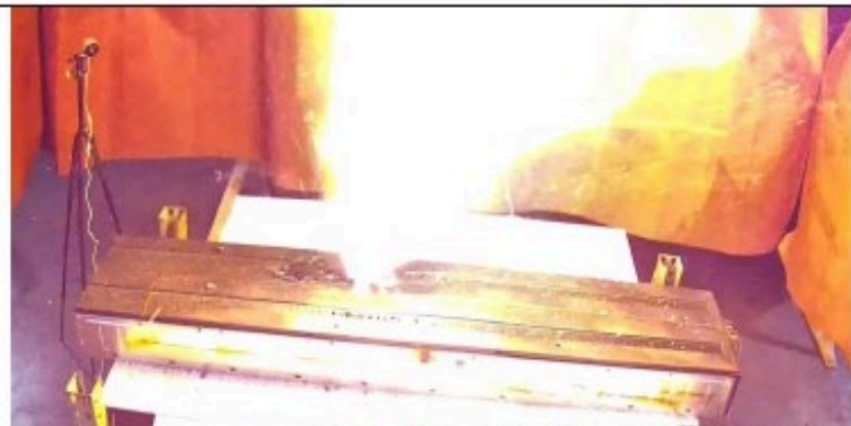
(g) First propagation after Initiating Cell (Cell 35) 00:58:04
