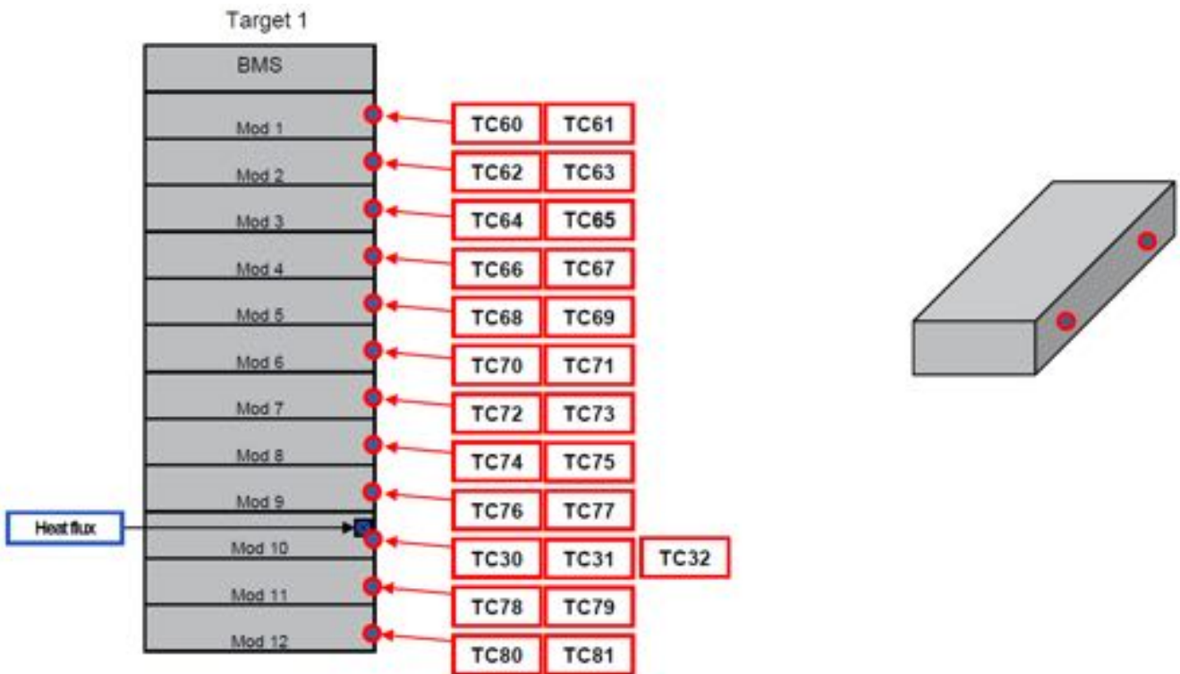
Figure C5 – Thermocouple and Heat flux locations in Target Unit 1
