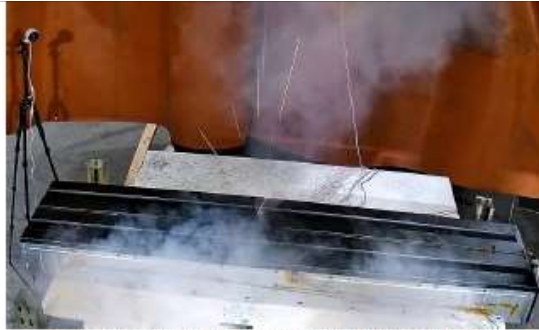
(c) Thermal Runaway (Initiating Cell) 00:46:14
