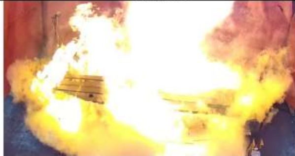
(e) Continuation of Initiating Cell Thermal Runaway 00:46:18
