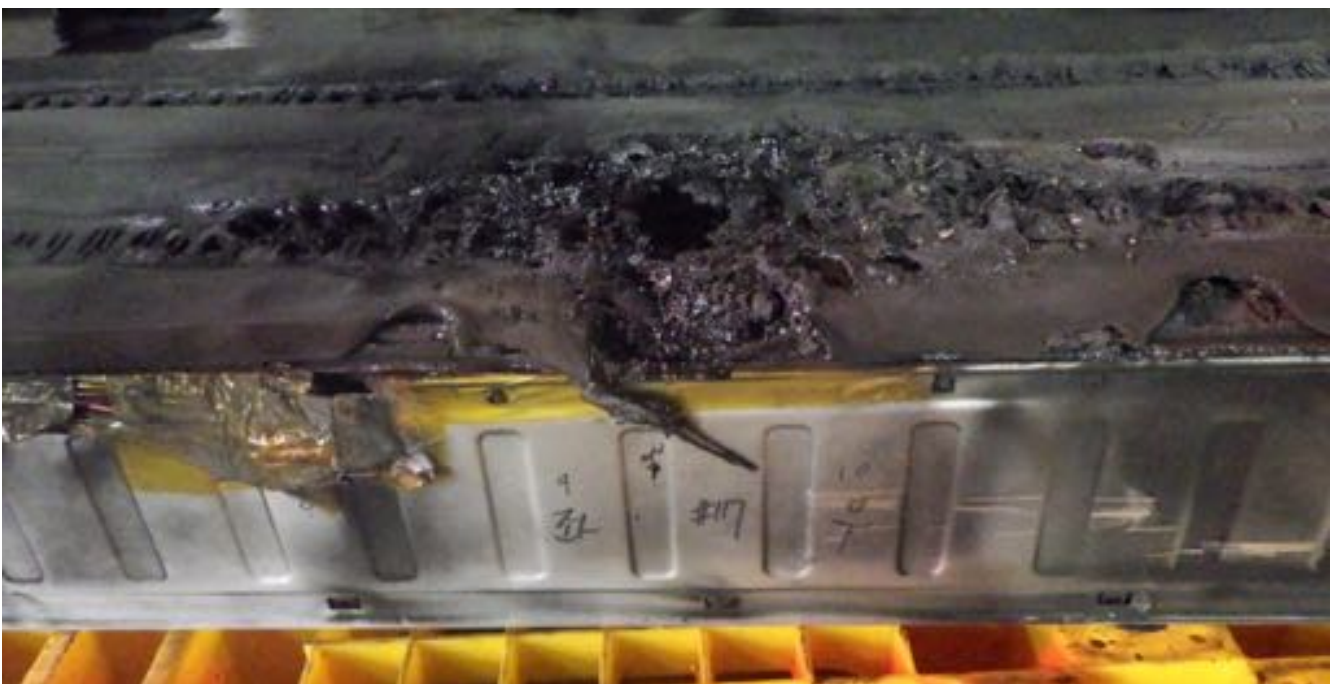
Figure E4 - Photo of the side of the initiating module after the test
