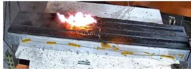
(f) Continued Flaming (post initiating cell thermal runaway) 00:46:41
