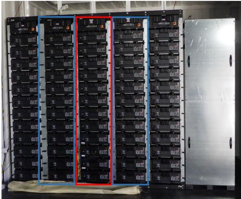
Figure B3 – Dummy units populated on the other side of the container (Initiating unit in red box and Target 1, 2 in blue box)
