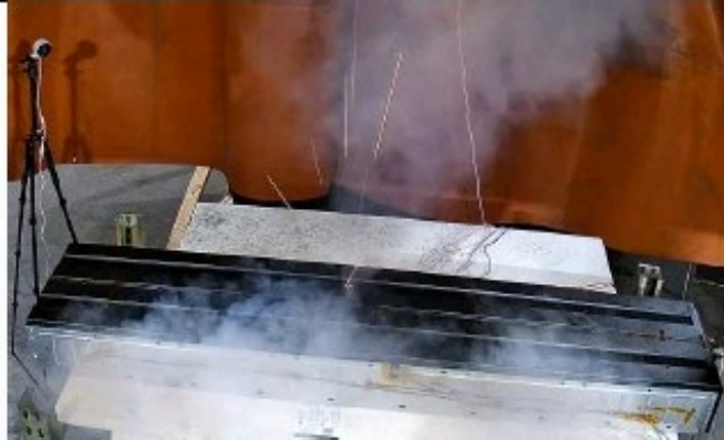
(c) Thermal Runaway (Initiating Cell) 00:46:14
