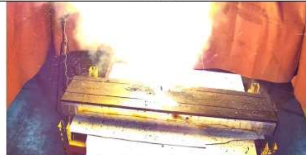
(h) Second propagation After Initiating Cell (Cell 31) 1:13:49
