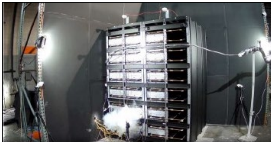
(c) Initiating Unit Thermal Runaway [00:42:25]
