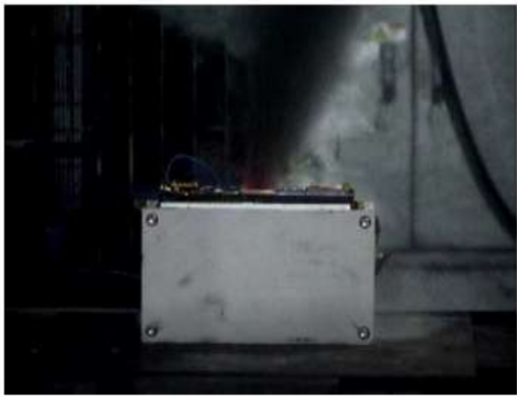
Cell 1 - Immediately before thermal runaway* (00:43:54)
