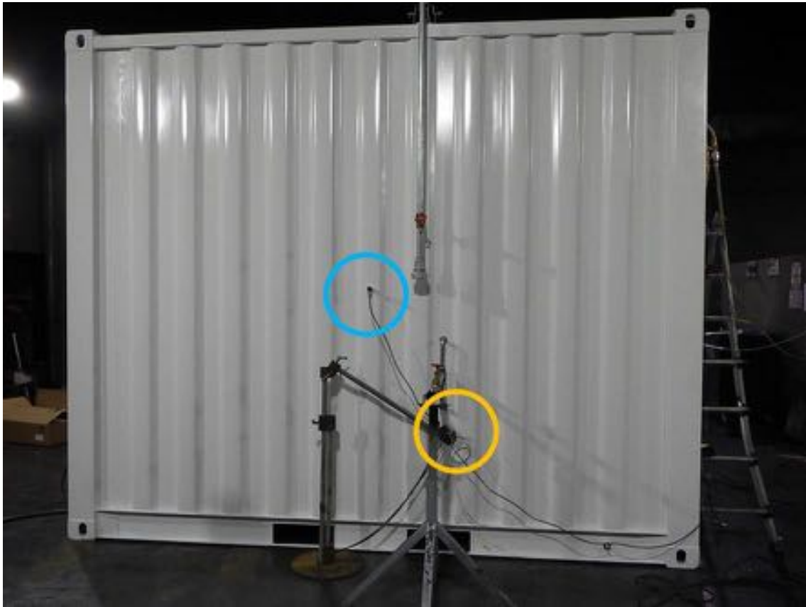
Figure C10 – Photo of the heat flux gauge (in the yellow circle) to account for the egress path and the pressure gauge to measure a potential explosion pressure (in the blue circle)
