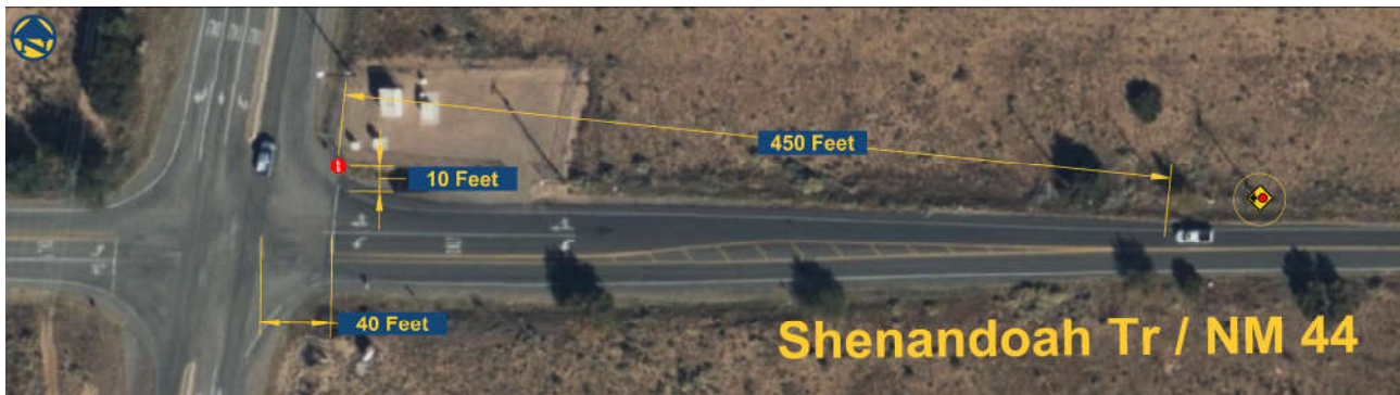
Figure 5: Existing Shenandoah Tr Westbound Approach Signage and Striping Measurements
