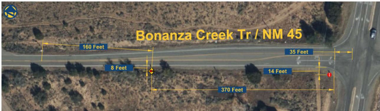
Figure 2: Existing Bonanza Creek Rd Eastbound Approach Signage and Stripping Measurements
